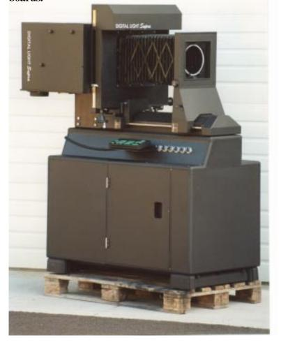
DeVere H810 chassis completely re-manufactured to new condition. All original DeVere electronics has been replaced with Durst and micro electronics, motor controls etc.
