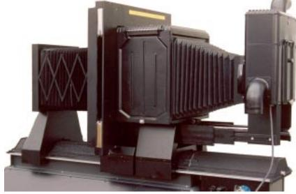
The lamp house is installed on a slider allowing the lamp to be focused for different focal length enlarging lenses.
