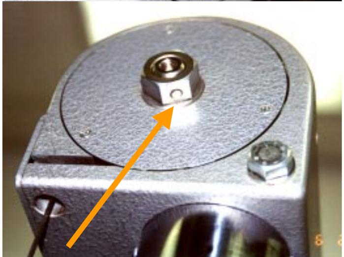
When the wire disk in the right side has been removed and the wire hanging loose it is possible to bring the tension tool back to a position where it is parallel with the column and then remove the “C” bracket.
