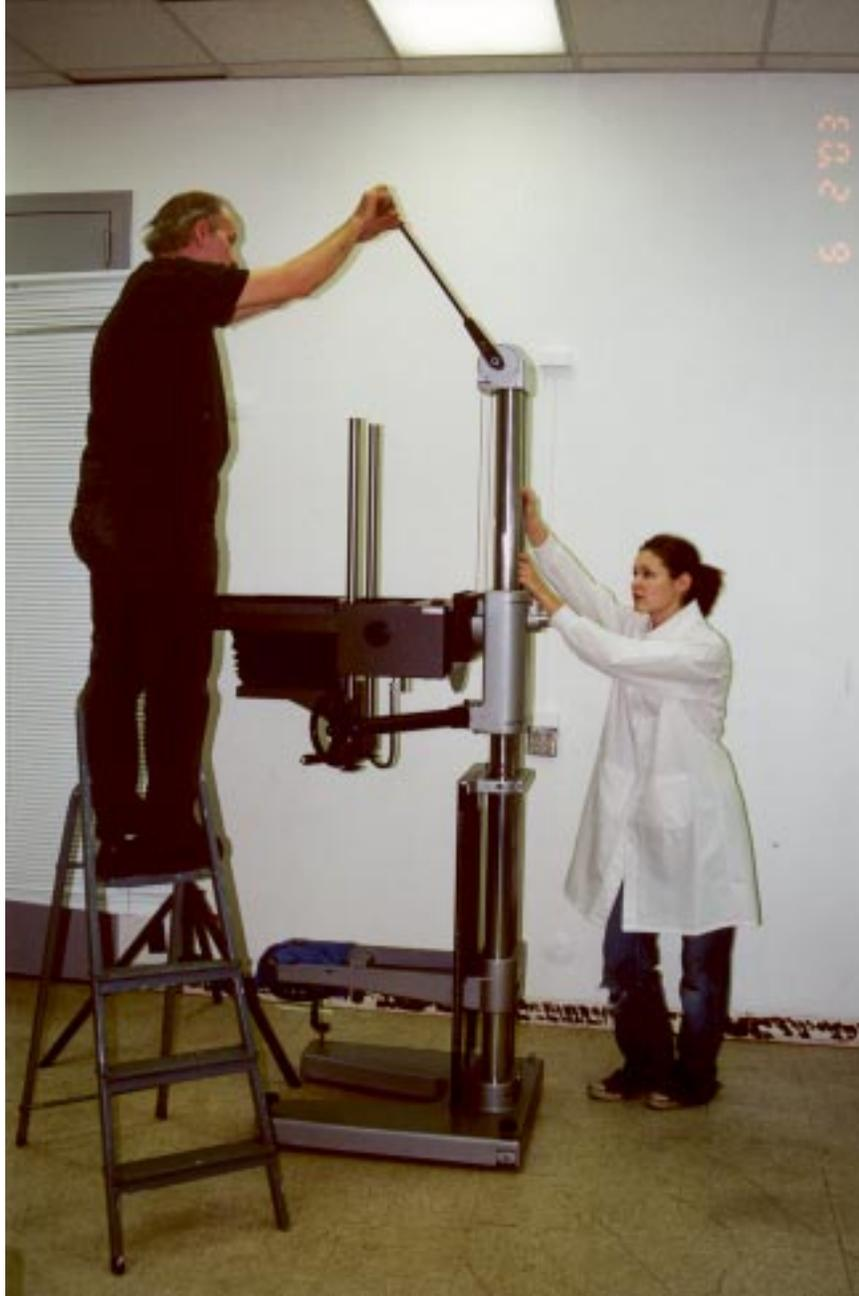
**This is the correct way to operate the spring tension tool. The person holding on to the chassis should be able to exert a force equal to lifting approx 50 pounds.**
