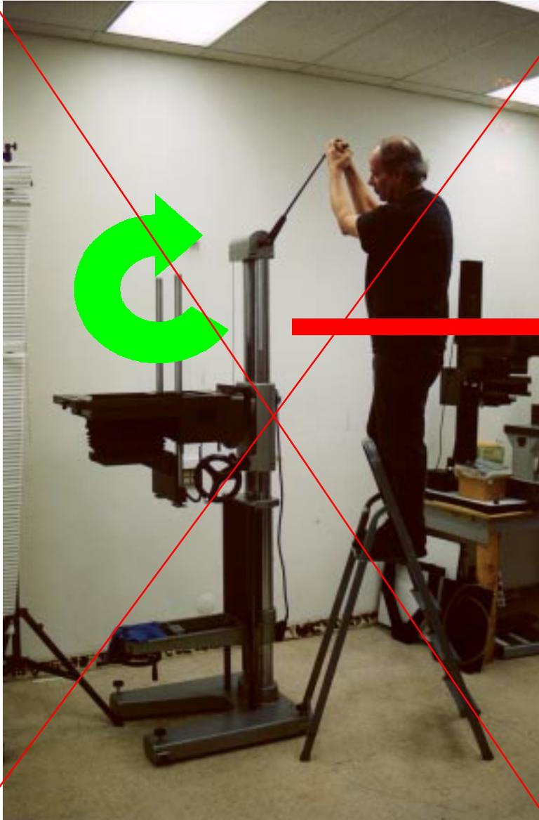
If this person continues the travel of the tool in a downwards direction the force of the spring will make the enlarger travel in the direction of the red arrow, as soon as you start the upwards motion. It will pull you of the ladder and possible hit you in the head with the end of the tool. The force released by the tension tool is several thousand pounds per square inch, enough to KILL if hit in the head or the face.
