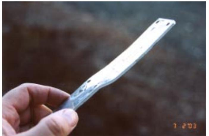
**If the spring is uncoiled uncontrolled it will crack the 1/2 to 1" thick cast aluminum housing**
