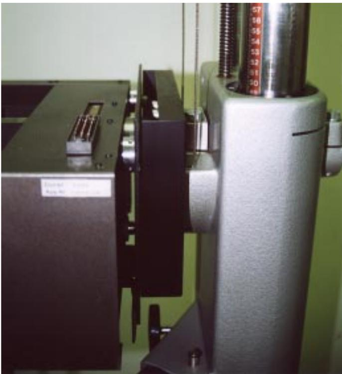
In order to remove the camera on an L184 it is only necessary to remove one screw. When this screw is removed the camera will slide off the support arm. Here it is also helpful to be two persons, one person to hold on to the chassis and one to pull the camera off. The camera is quite heavy, be careful not to drop it
