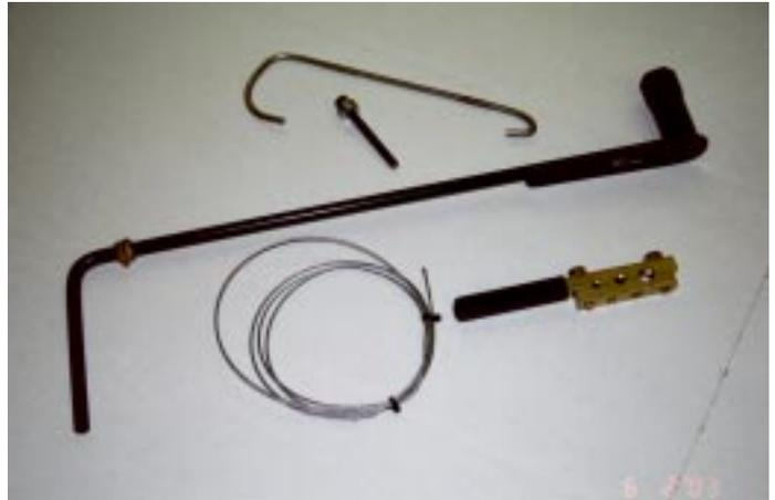
If a replacement wire has been ordered the wire kit will be enclosed with the tools. It is metric wire. It is important to use the right thickness wire,
