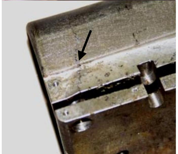
**On this picture you will see the effect of a spring accident. The force of the spring knocked the 1/2 - 1" thick aluminum housing almost 1/2 inch out of shape.**
