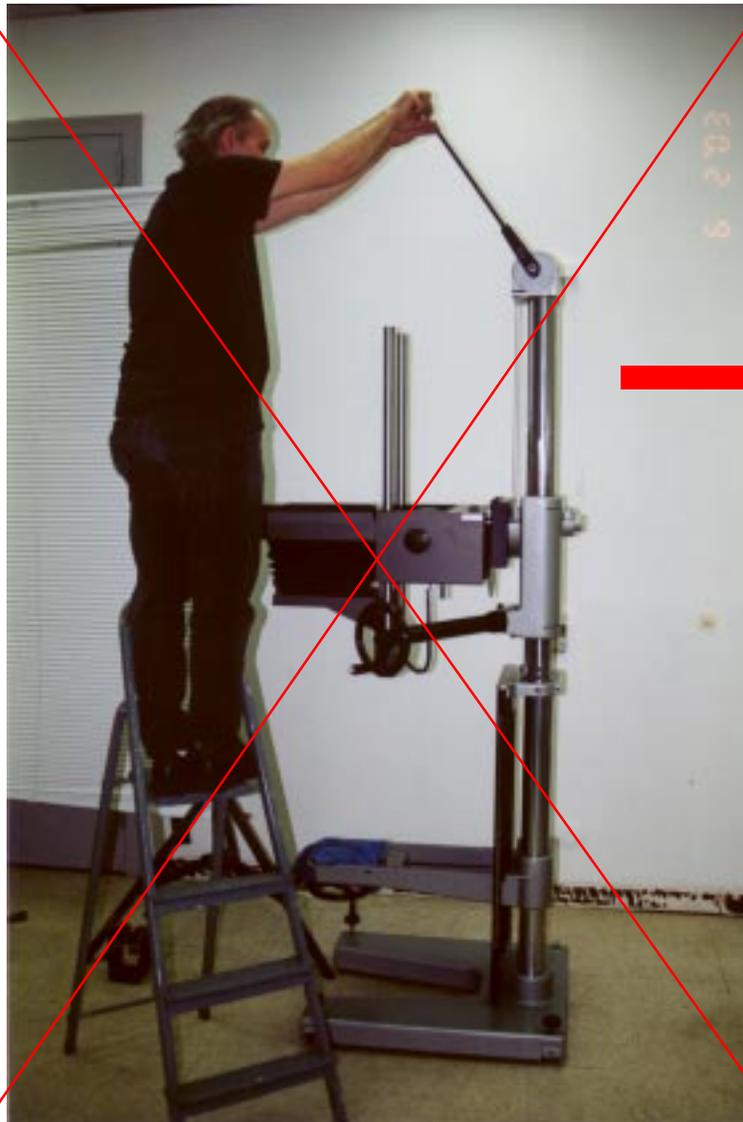
If this person continues the travel of the tool in a downwards direction the force of the spring will make the enlarger travel in the direction of the red arrow, it will pull you of the ladder and possible hit you in the head with the end of the tool. NEVER STAND IN THE LINE OF TRAVEL OF THE TENSION TOOL.
