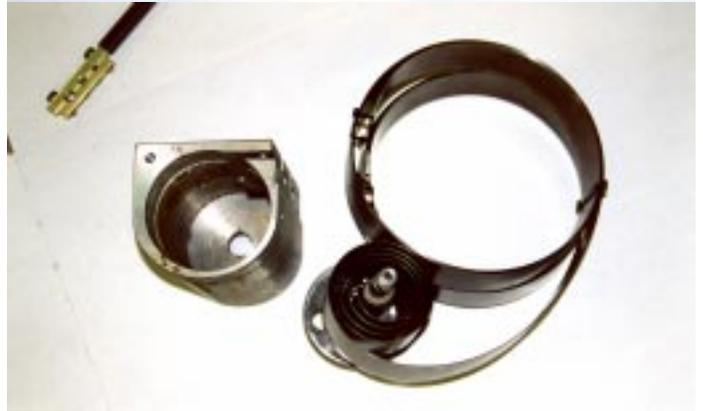
**The front plate on the spring housing is 4mm thick plate aluminum. If the spring is allowed to uncoil uncontrolled it will knock off this plate, ripping ALL SIX 4mm screws from their sockets.**
